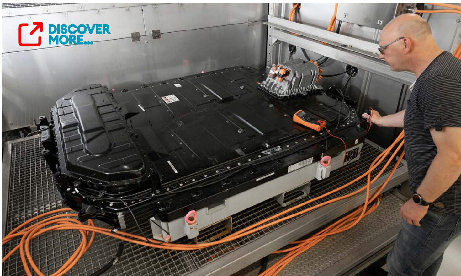
Audi invited us to see its battery testing facility in Germany where technicians can simulate a complete lifetime of use and abuse. Only when packs survive the equivalent of 15 years of charging and driving are the designs approved for production
